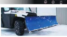
PLOW IS AUTOMATICALLY RAISED WHEN SHIFTING INTO REVERSE
