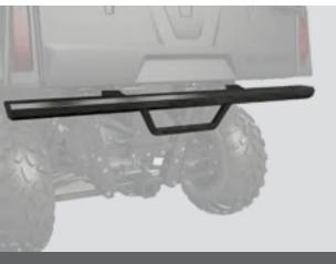
**1 ¼" DIAMETER** STEEL TUBE CONSTRUCTION
